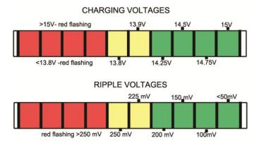
Low charging voltage: Check belts for slippage. Check connections from the alternator to the battery. If no problems are found, replace the alternator.
